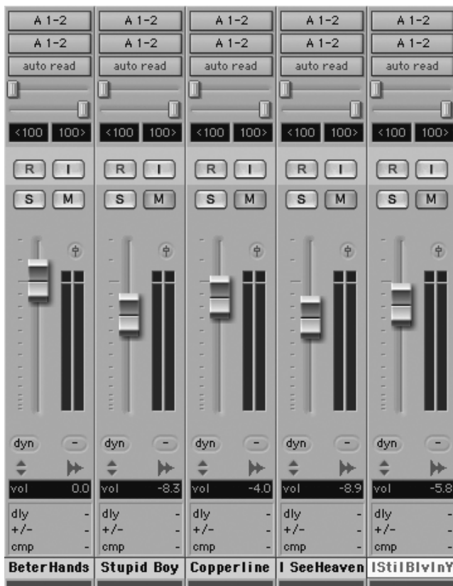
Figure 10.2 Carefully match the levels of your reference songs to the level of the song you're mastering.
