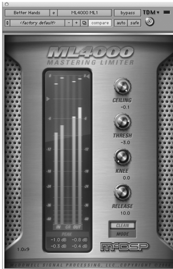
Figure 10.4 Using a limiter to add 3 dB of level to the track with minimal gain reduction.
